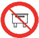
**Advise the customer that if the GAS system fuse burns, the connections of the devices to which it is connected will be restored. It is strongly recommended not to replace the fuse with another one with a higher amperage rating since it may cause irreparable damage.**
