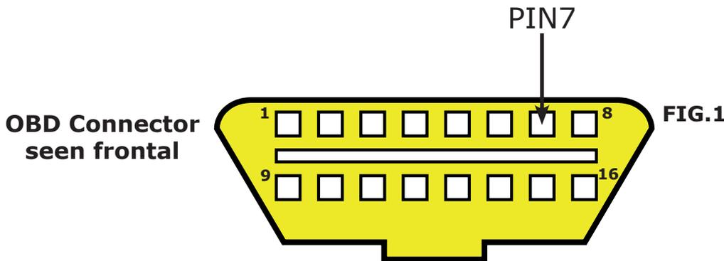
Connect the GREEN wire to the signal found on PIN 7 of the OBD connector.
