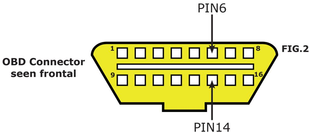
Connect the YELLOW-GREEN wire to the signal found on PIN 6 and the wire YELLOW-GREY to PIN 14 of the OBD connector.
