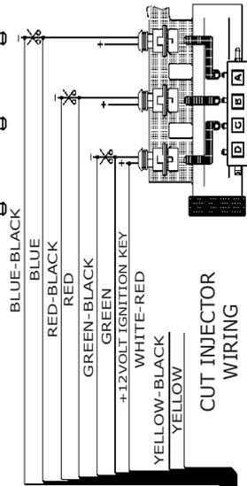
**INTERRUPT THE INJECTOR NEGATIVE WIRES.**
