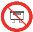
**Advise the customer that if the GAS system fuse burns, the connections of the devices to which it is connected will be restored. It is strongly recommended not to replace the fuse with another one with a higher amperage rating since it may cause irreparable damage.**
